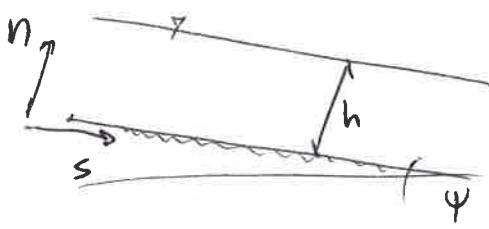
$$\left\{ \begin{array}{l} \frac{\partial}{\partial t} (\rho h) + \frac{\partial}{\partial s} (\rho v h) = 0 \\ \frac{\partial}{\partial t} (\rho v h) + \frac{\partial}{\partial s} (\rho v^2 h) = -\frac{\partial P}{\partial s} + \rho g h \sin \psi - T_0 \\ T_0 = \rho g h \cos \psi \cdot \tan \psi + \rho g \frac{v^2}{2} \end{array} \right.$$
