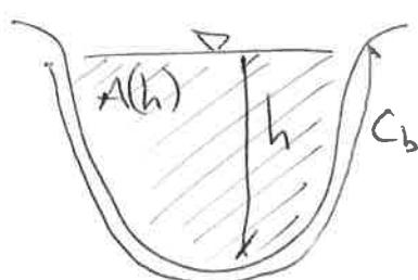
$$\frac{\partial}{\partial t}(\rho U A) + \frac{\partial}{\partial x}(\rho U^2 A) = \gamma A \sin \psi - \frac{\partial P}{\partial x} - \bar{T}_0 \cdot C_b$$
